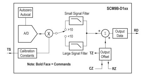
SCM9B-D134 Block Diagram - For Module Dimensions and Pinouts, See Page 5-26
