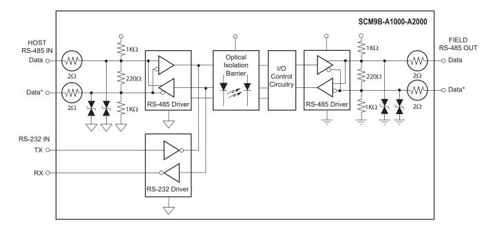
SCM9B-A1000/A2000 Block Diagram - For Module Dimensions and Pinouts, See Page 5-26
