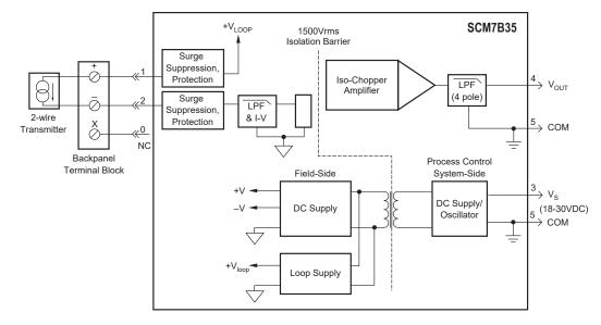
SCM7B35 Block Diagram - For Module Dimensions and Pinouts, See Page 2-26
