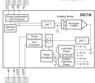
DSCT36 Block Diagram - For Module Dimensions and Pinouts, See Page 7-47
