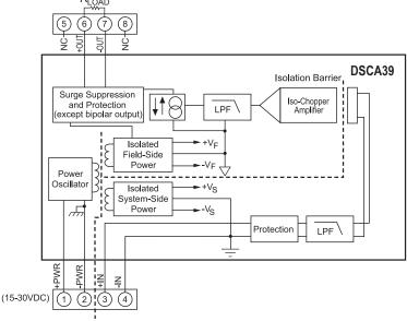
DSCA39 Block Diagram - For Module Dimensions and Pinouts, See Page 4-35
