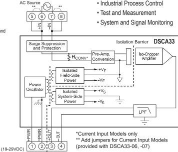
DSCA33 Block Diagram - For Module Dimensions and Pinouts, See Page 4-35
