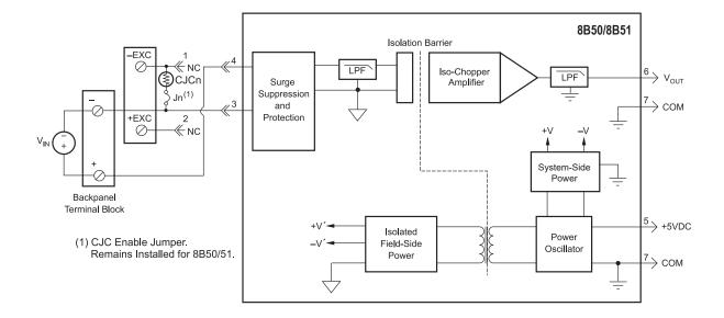
8B50/51 Block Diagram - For Module Dimensions and Pinouts, See Page 3-40
