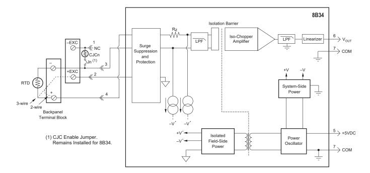
8B34 Block Diagram - For Module Dimensions and Pinouts, See Page 3-40
